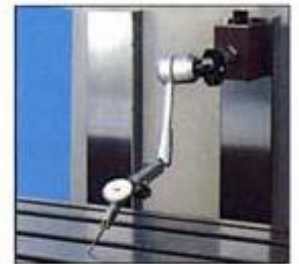
0.015/500mm(0.0006"/20") Parallelism of Table Movement In-x-axis
