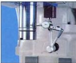
0.01mm/127mm(0.0004"/5") The Accuracy of Travel of Main Spindle Quill
